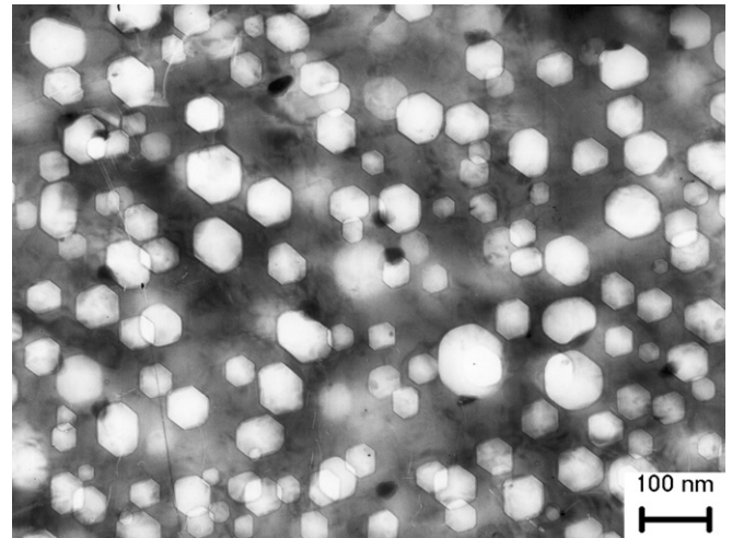
Fig. 5. Voids and G-phase precipitates observed at the core center plane cross section of fuel pin #18 cladding.
